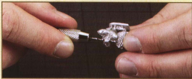
Drill a hole through the hand with a pin vice.
